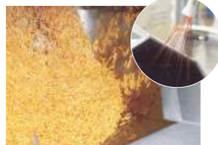
The crackers are then seasoned with our secret sauce. The crackers are rotated when seasoned so the taste is uniform and the crackers become glossy.
