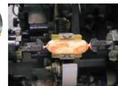
The crackers are wrapped up like sweets at a high speed of 300 pieces per minute.
