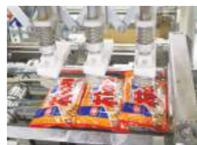
The crackers are placed in little bags with peanuts. A puff of nitrogen gas is used to protect the product and with that, the process is complete!
