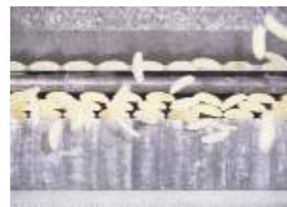
A high speed cutter is used to cut the chilled dough to a half moon shape with the thickness of around 1.6mm. 1,500 Kakinotane are cut every second!
