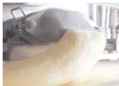
Rice flour is steamed at a high temperature and then kneaded to make the dough. Around 300kg of dough can be made at one time!
